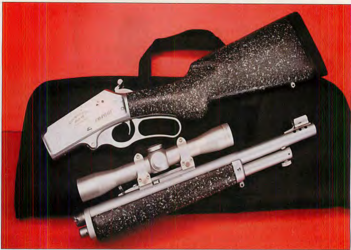
The Alaskan CoPilot (above) shown with optional Kevlar stock, hard chrome finish and scout scope system. This take-down rifle conversion comes in 16.5, 18.5 or 20-inch barrel length. (left) Brown was pleased with his group at 50 yards "I even had a witness," he chuckled. He went on to say, "I reckon this is good enough for government work."
